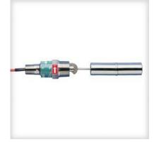
These units solve the problem of **point level sensing** in tanks with inaccessible tops or bottoms, or at intermediate locations in larger tanks. Operation is positive and dependable. The float pivots with changing liquid level, displacing a shuttle which magnetically actuates a hermetically sealed switch within the unit. Installation is through the tank side at the detection point. **LS-52100 : Rugged, all stainless steel unit offers a broad chemical compatibility at temperatures to 150°C.**
